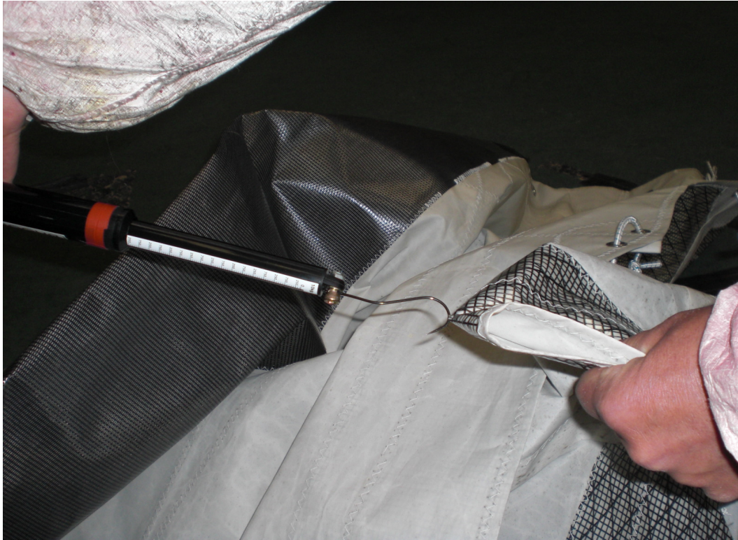
Fig 6. Hook through one spanwise cord which is woven under the surrounding cords as shown. Allow the sail to fold and grasp both surfaces. Pull gradually up to the test load as shown.
